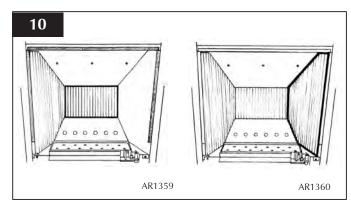
8.3 Locate the top panel on top of the sides and rear by lifting it up and forward inside the box, Then sliding it backwards and down behind the side panels and to rest on the rear panel. See diagram 11.
